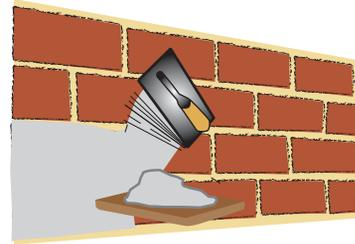
If you are applying more than one coat, you will need to let each coat dry for at least 3 - 7 days. You will then need to scour each coat with a sharp object to provide a good surface for the second coat of render to bond to.
